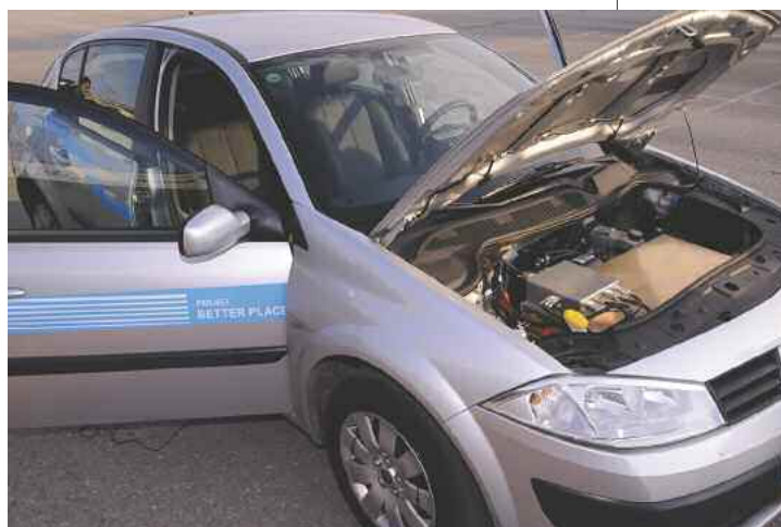
A Better Place prototype electric car. Better Place and Renault-Nissan plan to deploy hundreds of test cars, thousands of charge spots, and several battery-swap stations in Israel by late 2009.
